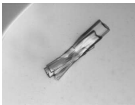
Figure 2 A cluster of gankyrin crystals with approximate dimensions 1 \times 0.2 \times 0.07 \text{ mm} . A single crystal was cut from this cluster and used for data collection.
